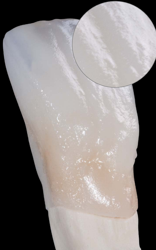
Surface structure of the monolithic crown
